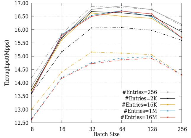
Figure 5: The effect of batch-size  $B$  on application throughput, for five different configurations of the L2 forwarding application. The solid line represents  $b = B$  (sub-batching enabled), and the dotted line represents  $b = 1$  (sub-batching disabled).
